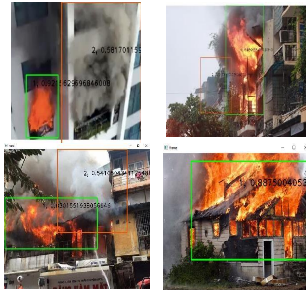
Fig. 9. Visualization results on some images of test dataset. Fire areas are box-bounded by green rectangles with number “1” and confidence score, the smoke areas are box-bounded by red rectangles with number “2” and confidence score.
